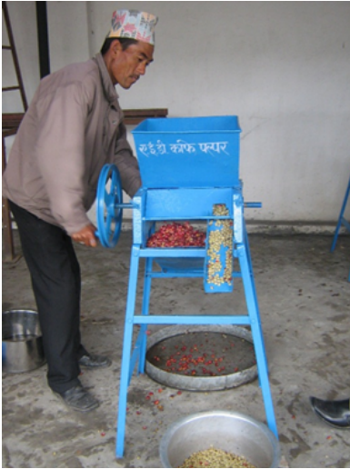
Fig 2. Hand operated coffee pulper
